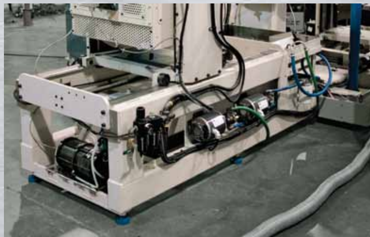
Air/oil booster for stall brake and linear adjustment. Shown along side fluid fill and evacuation system.
